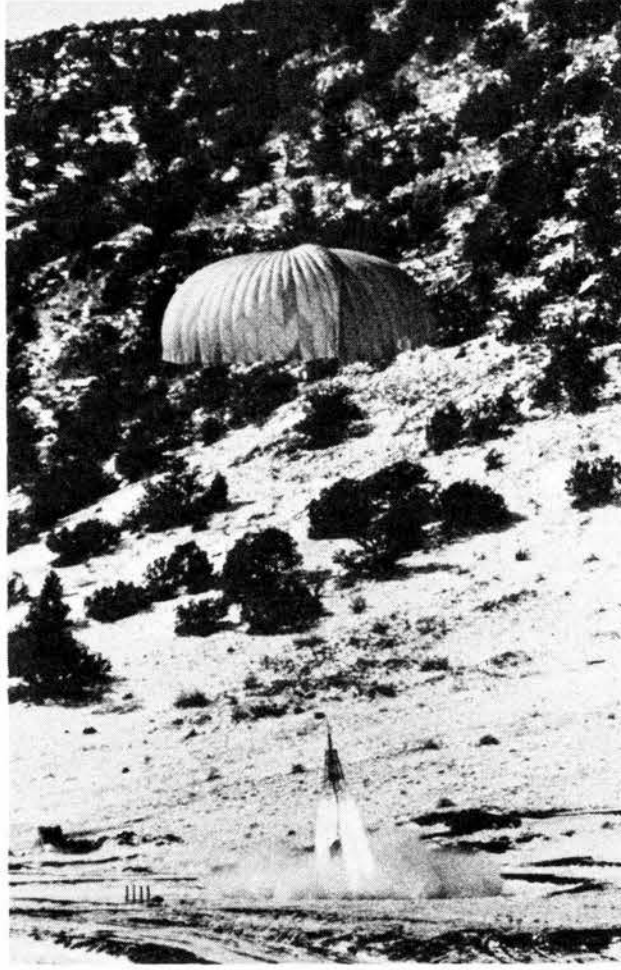
RETROROCKETS OF THE RAPID system stopped a 5000-pound sphere in mid-air and gently lowered it to impact during a drop test recently from the Sol Se Mete aerial cable facility in Coyote Test Field.
